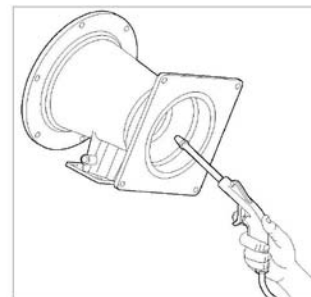
Fig. 30 Venturi being cleaned with compressed air
