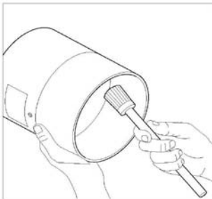
Fig. 29 non return valve being cleaned with soft brush
